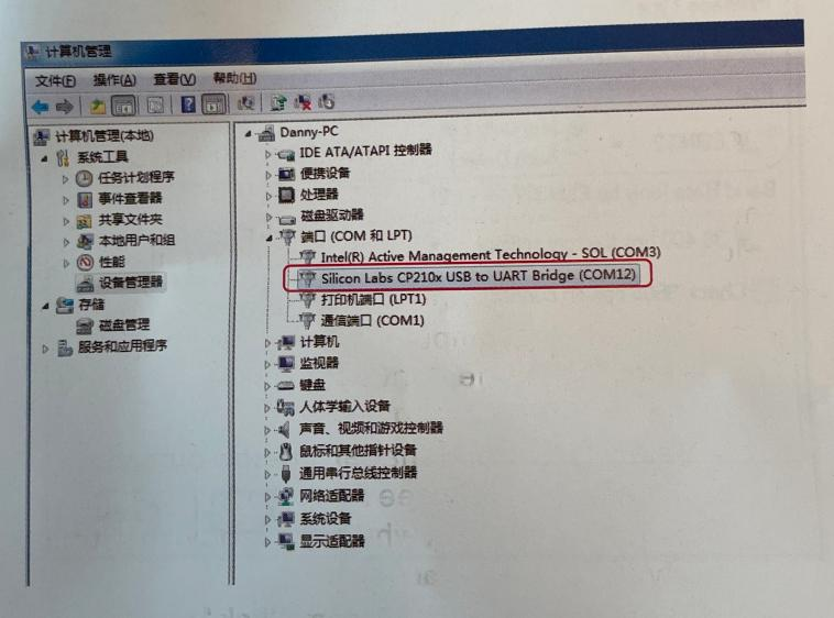
3. Run ScanMaster-ELM below Options-Communication, choose Serial (RS232 or Virtual COM Port Driver) for icon , set serial port number manually with the number which is the same in last step.
